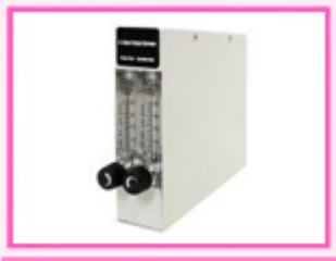
N 2 Autoflow system The autoflow system is developed to use in combination with a drying cabinet. The device is used for the quick removal of moisture in the cabinet after the doors have been opened. The drying process is realised by using Nitrogen (N 2 ), which is purged automatically after the doors are closed. (timer controlled)
